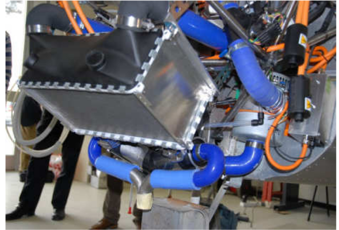
Figure 6. Installed heat exchanger and cyclone unit.
