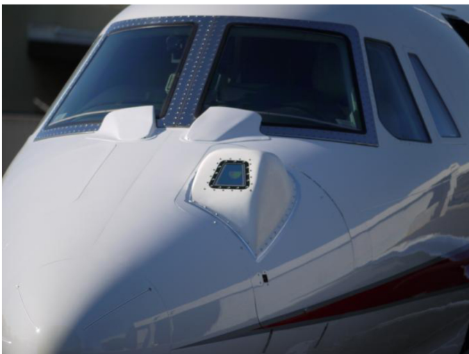
Figure 1. Installation of Kollsman EVS II camera on the Cessna Citation Sovereign
