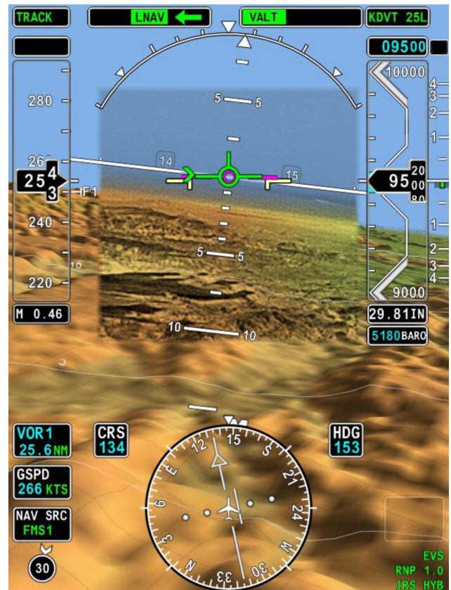
Figure 3. Honeywell CVS showing the colorized the IR image inside the center window of the SVS display
