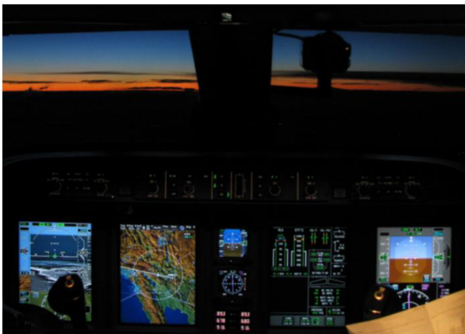
Figure 2. CVS integrated on Sovereign Flight Deck
