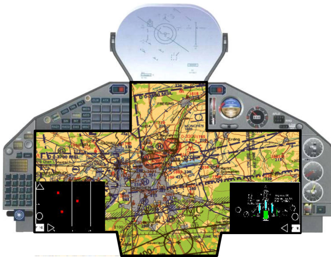
Figure 2. Cockpit Configuration with the Panoramic Display
