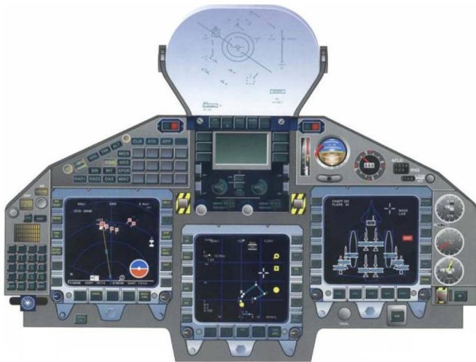
Figure 1. Traditional Cockpit Configuration with three Head Down Displays
