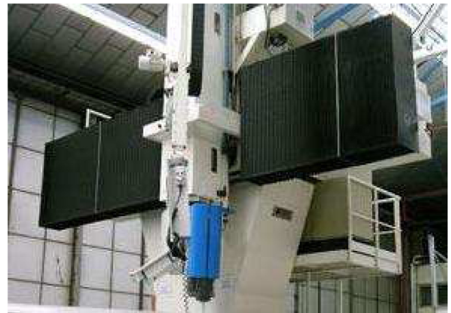
Figure 1. SPIE end effector on cartesian machine (2002)
