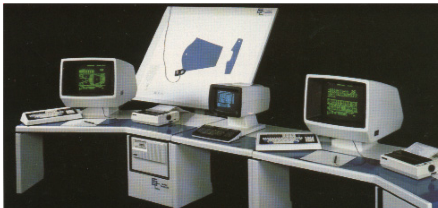
Figure 3. Automated Gerber-marker making system.
