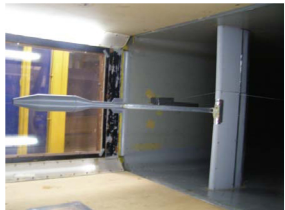
Figure 2. Test Section Sting Mount. The baseline model was mounted on a sting which attached to a three component balance below the test section.
