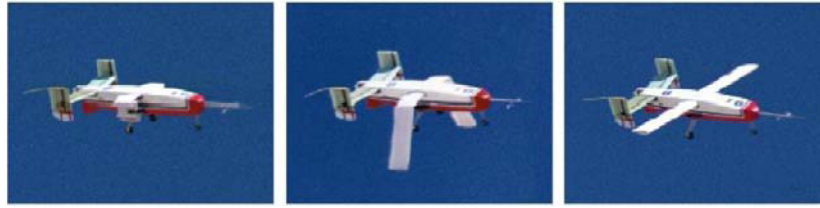
Figure 1. Previous Transforming UAV Research. The NASA Dryden I2000 with inflating wings was presented in “Aerostructural Interaction and Optimization of Inflatable Wings.”[10]
