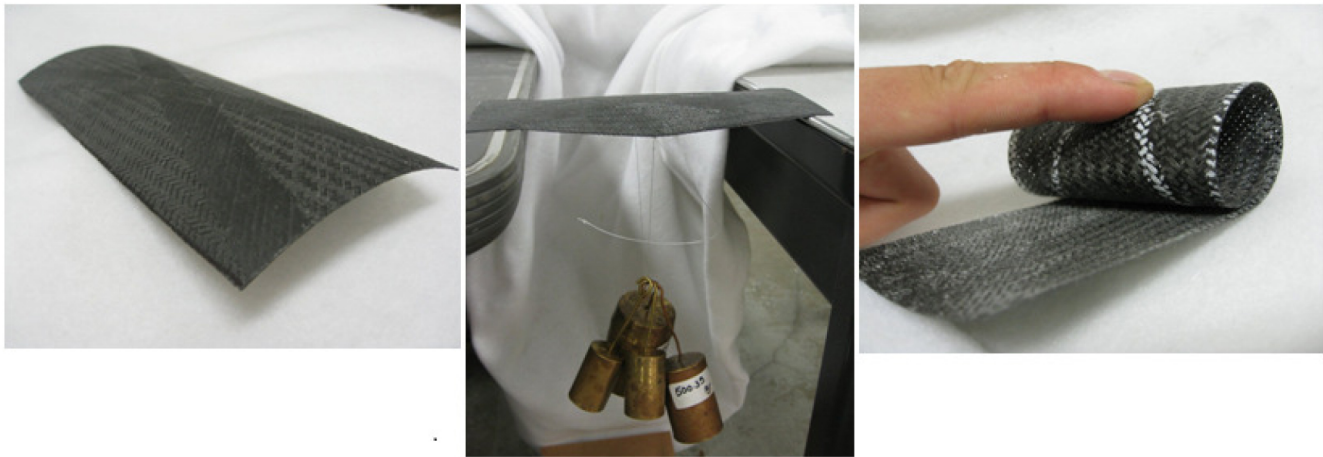
Figure 1. Tape Spring Behavior, Left: Normal Deployed, Middle: Loaded, Right: Rolled
