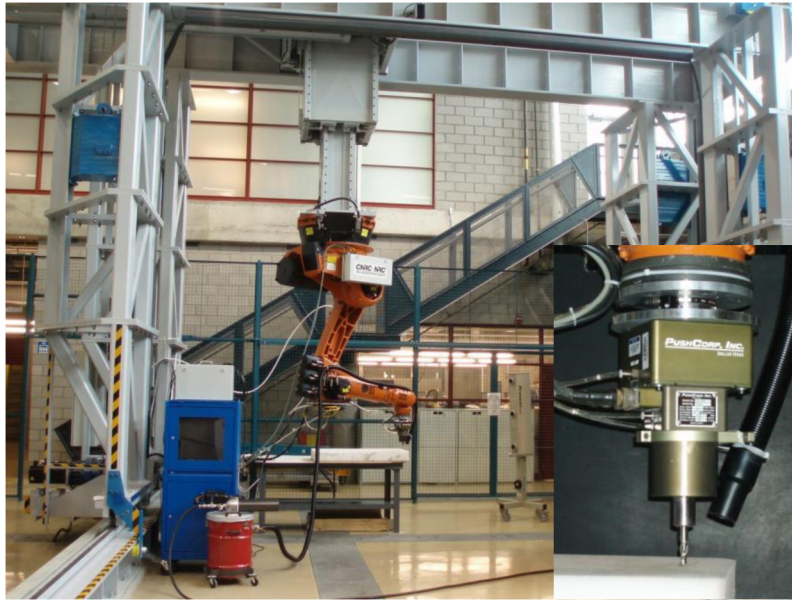
Figure 2. Robot-Mounted Gantry System and Spindle
