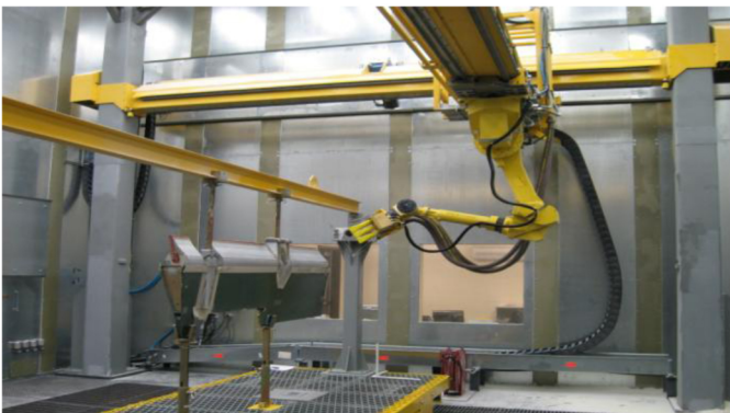
Figure 1. Gantry Robot Developed by SwRI for Off-Airframe Component Paint Stripping
