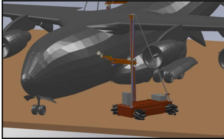
Figure 3. Concept for a Mobile Robotic Platform for Large Aircraft Depaint
