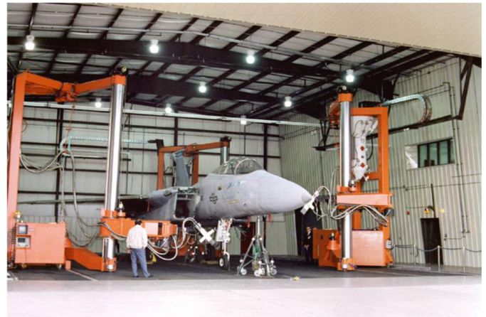
Figure 2. Free-Standing Robots Developed by SwRI for F-15 Paint Stripping
