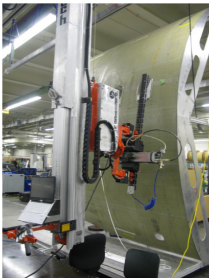
Figure 3. Handling system loading machine on fuselage assembly
