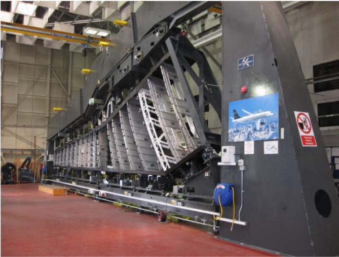
Figure 1. C-Series Demonstrator Wing Box Jig, Belfast
