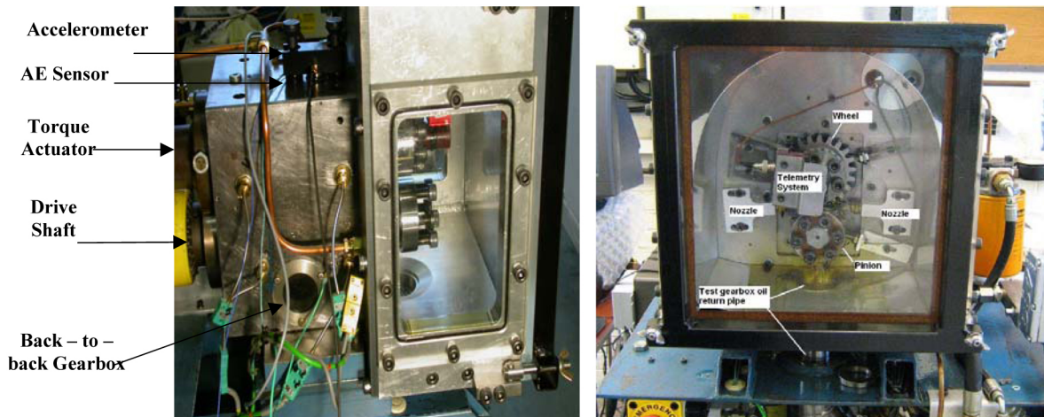
Figure 2. The 75 mm centre distance back-to-back gearbox
