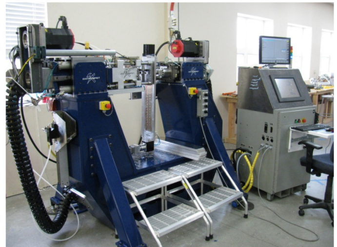
Figure 1. Automated squeeze riveting machine utilizing the coaxial head design
