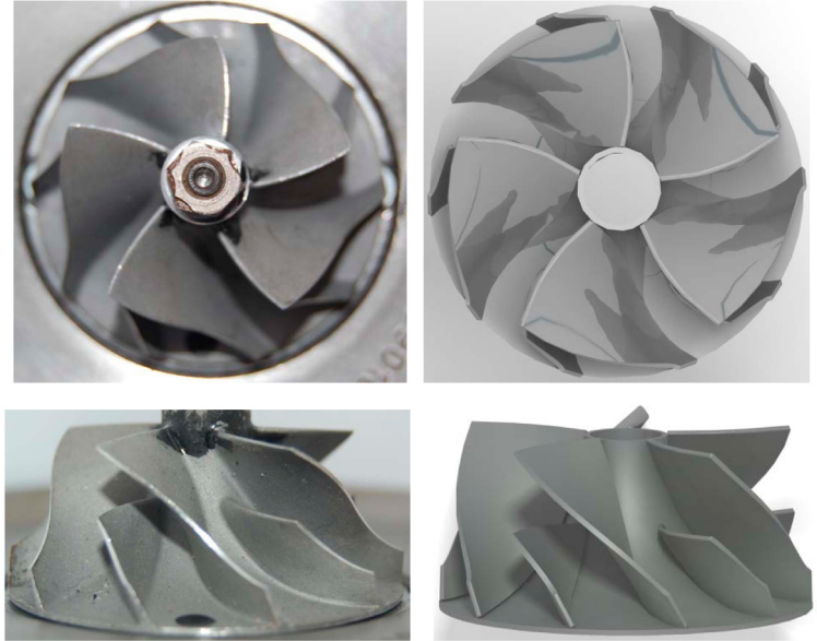
Figure 2. Actual impeller geometry (IHI RHF3 compressor) and related 3D reconstruction
