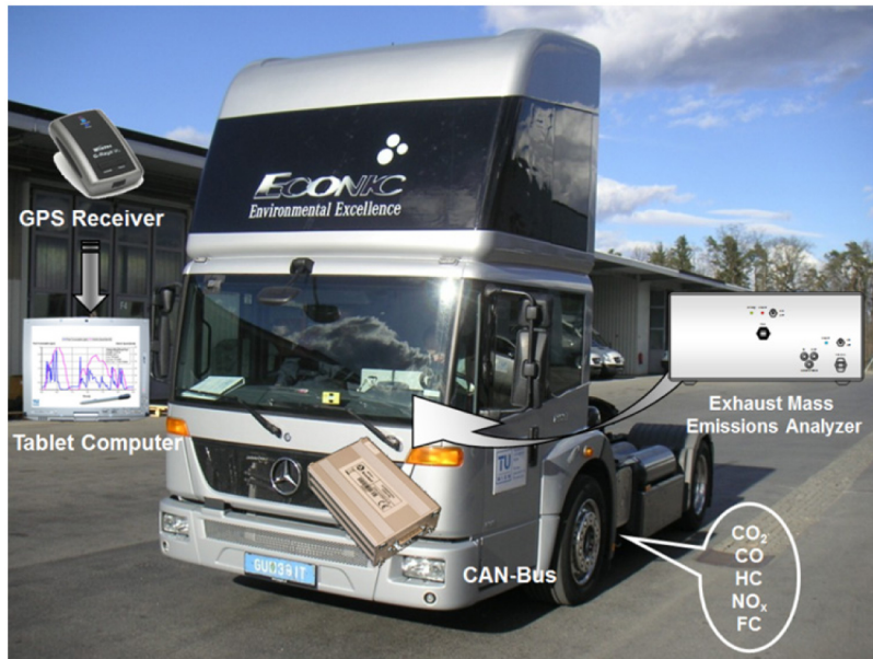
Figure 2. Detail of the PEMS installed in the test vehicle.
