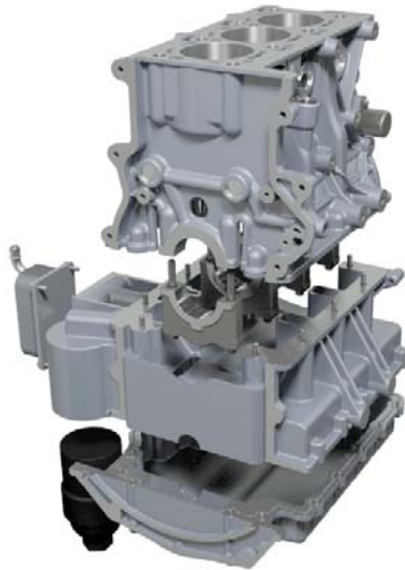
Figure 6: cylinder block structure: Aluminum low pressure casting with fracture split main bearing inserts [4]
