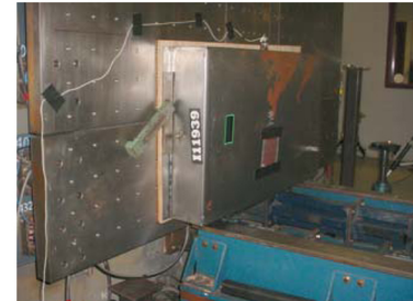
(c) Steel box with a LHS hole.
