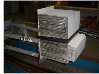
(c) Deformable impactor.
