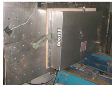
(b) Steel box with a RHS hole.
