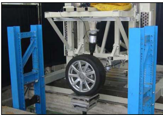
Figure 8. IAE quarter vehicle test rig
