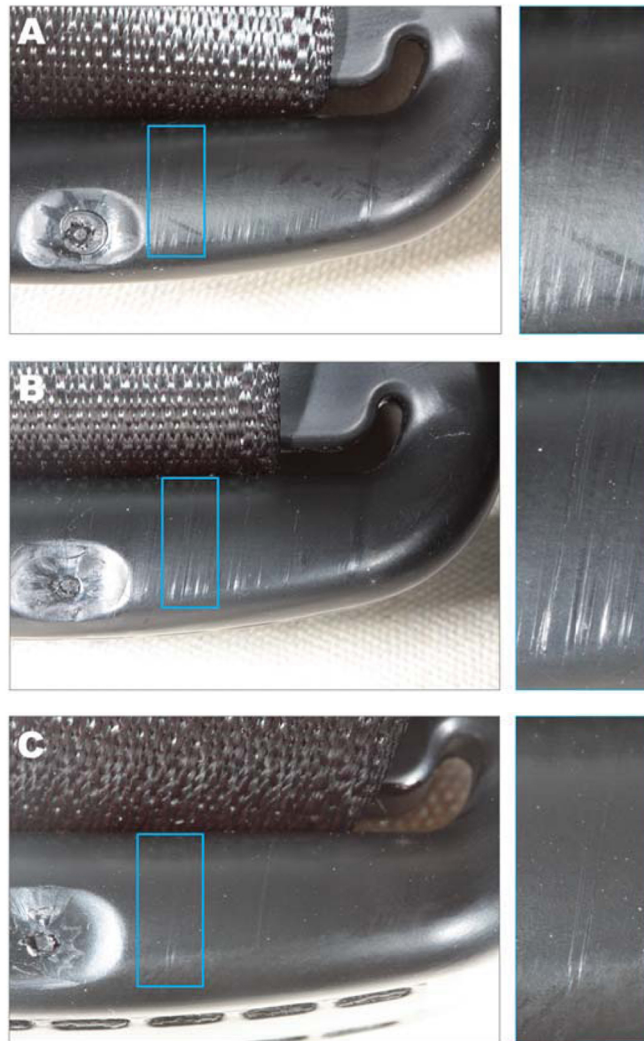
Figure 9. D-ring abrasions generated by tempered glass fragments - (A) Small [Test G3], (B) Intermediate [Test G1], (C) Large [Test G2]
