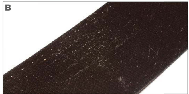
Figure 8. Baseline test B1 results - body side of latch plate (A) and corresponding webbing (B)
