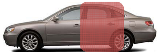
Figure 2. Direct Impact - Direct damage overlaps proximal to occupant seat position.
