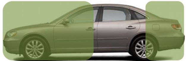
Figure 1. Direct damage does not overlap proximal to occupant seat position.
