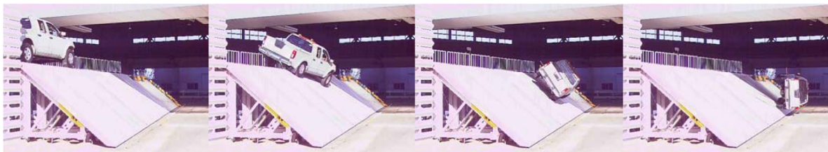
Figure 2. Ditch fall-over test
