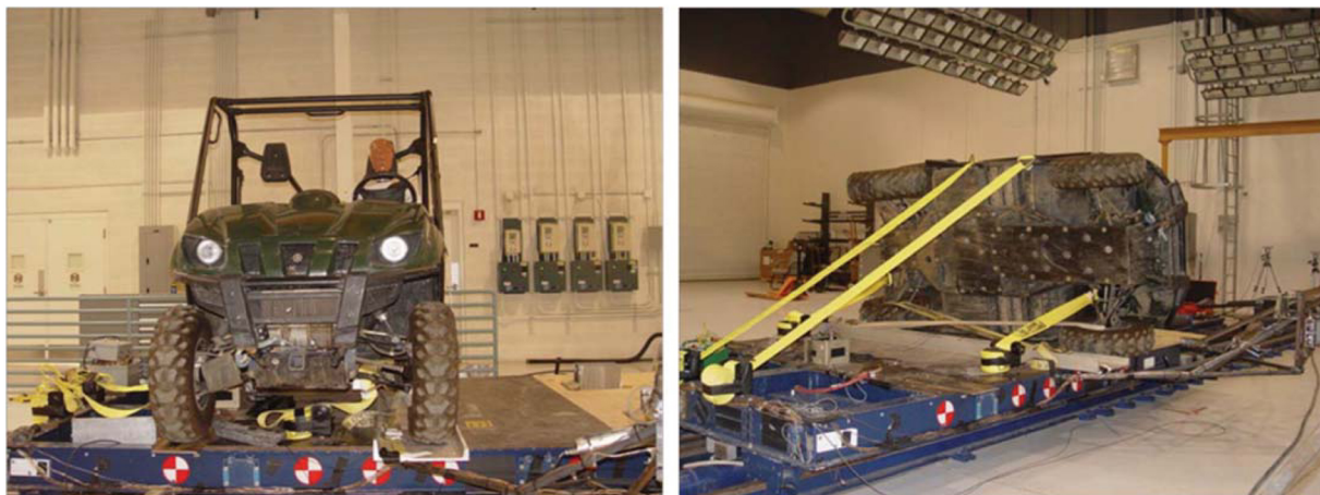
Figure 1. Deceleration sled test configuration for driver-side-leading tip-over simulation.
