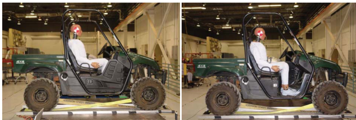
Figure 2. Photographs of unbelted ATD occupant in ROV with (left) and without (right) a sculpted door present.
