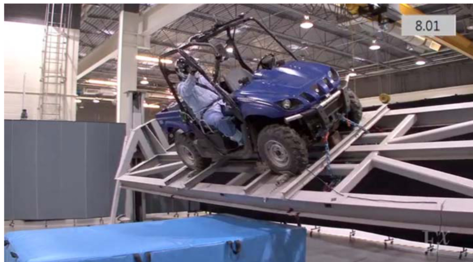
Figure 6. Video frame from passenger roll spit during quasi-static roll to 90-degrees. This is the 95 th -percentile male volunteer in the one-handhold configuration.
