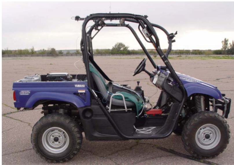
Figure 3. Vehicle setup for active occupant response testing.
