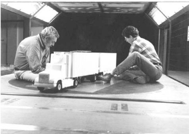
1b). skirts being fitted to the 1:10-scale model. Fig. 1. Installation of the Model in the NRC 2m × 3m Wind Tunnel.
