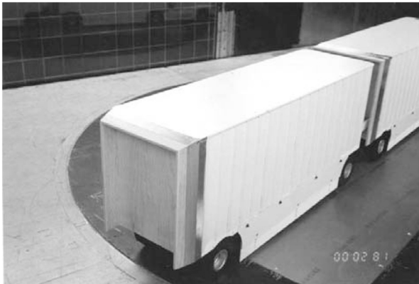
4b). tandem trailers, 15° rear and 0° front triple boat-tail panels
