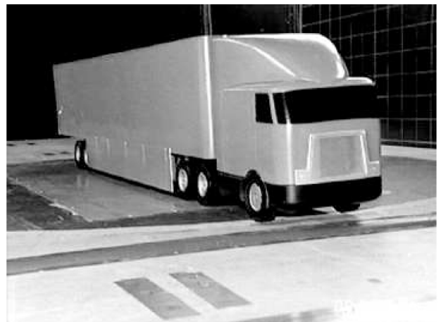
3b). preliminary skirts at 152 mm clearance Fig. 3. Navistar COE Tractor and 14.6 m Single Trailer.
