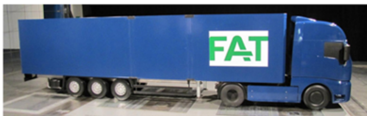
Figure 4. Complete wind tunnel model on a scale of 1:2.5 of the generic truck
