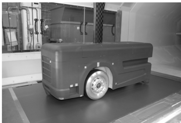
Figure 2. The truck model mounted in the Chalmers wind tunnel L2.
