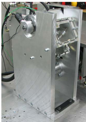
Figure 4. Fully functional single valve train mock up
