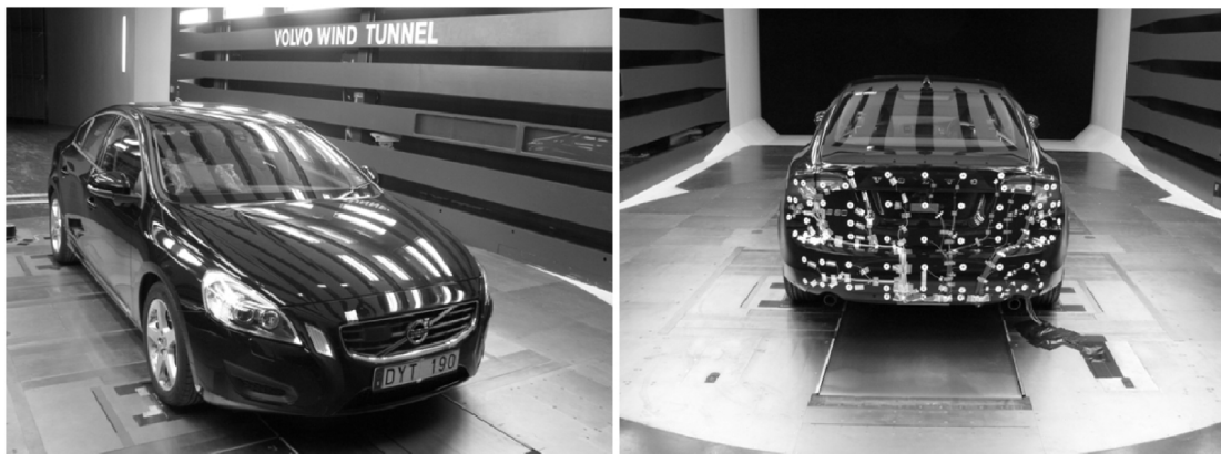
Figure 1. Overview of the wind tunnel model with base pressure measurement set up to the right.
