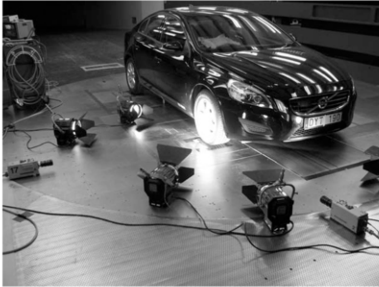
Figure 3. Set up of high speed cameras and spotlights for tire geometry investigation.
