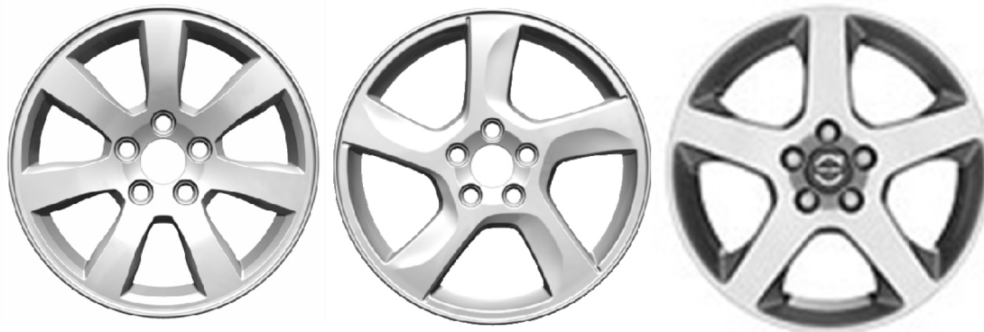
Figure 4. Overview of wheel design, denoted Wheel 1- 3 from left to right. Wheel 1 is 16" and Wheels 2 and 3 are 17".
