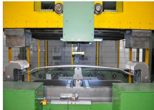
Figure 13. The leaf spring exposed to strain during the shot peening process
