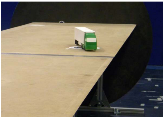
Figure 6. Vehicle model behind on the flat plate during wind tunnel tests.
