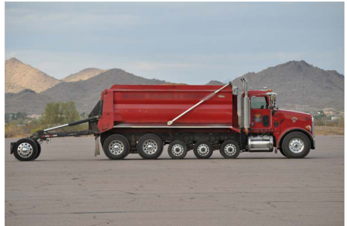
Figure 4. Test Vehicle: Heavy Duty Dump Truck with Trailing Axle.
