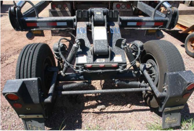
Figure 1. Articulated design trailing axle.
