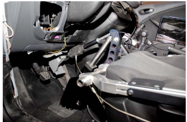
Figure 4. Image of the brake pedal of the robot mounted in the car (source IDIADA)
