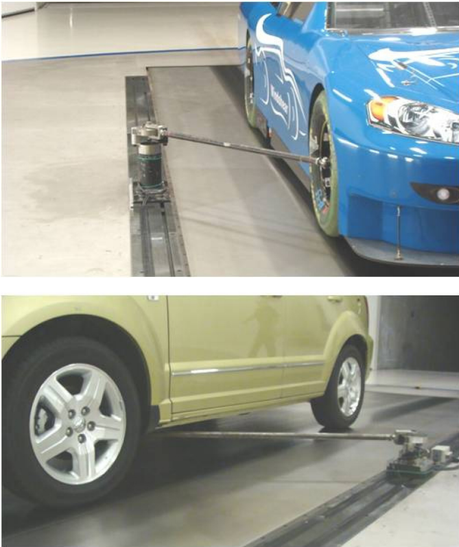
Figure 14. Typical restraint locations for NASCAR vehicles (above) and production vehicles (below)
