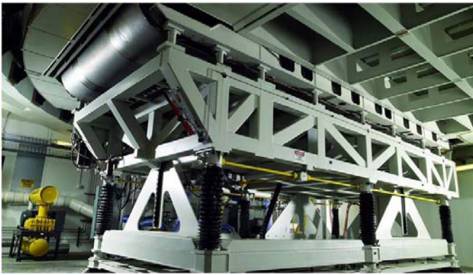
Figure 6. Windshear wide-belt moving ground plane viewed from below the test section
