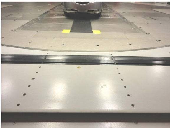
Figure 4. Primary suction scoop and secondary suction and blowing slots
