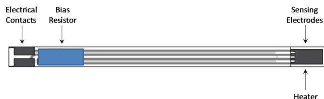
Figure 5. Particulate Matter (PM) Sensor Sensing Element (Enlarged)
