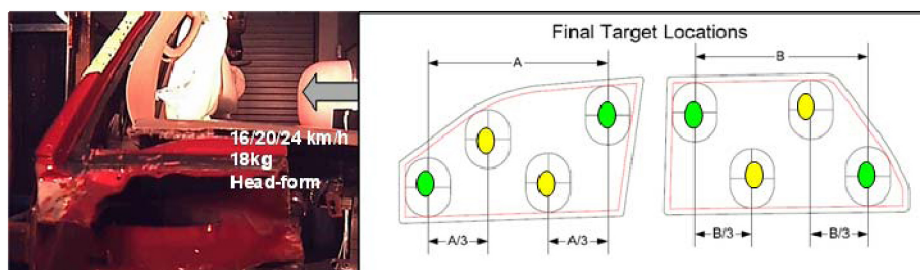
Figure 1. NHTSA Ejection Mitigation Research Component Test Setup.
