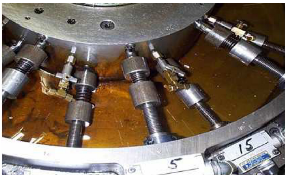
Fig. 4. Rotary cycle tester [4]
