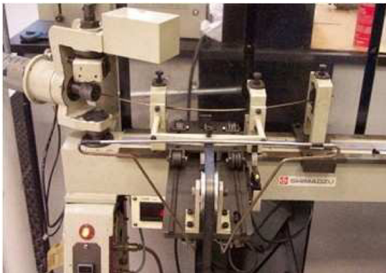
Fig. 3. Nakamura rotating bending tester [4]
