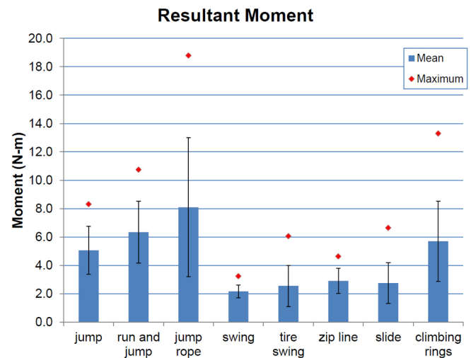
Figure 5. Mean and maximum resultant moment. Results shown are mean \pm standard deviation. Maxima are shown as red diamonds.
