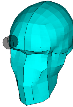
Figure 3. Frontal bone impact test simulation of Cormier test setup.
