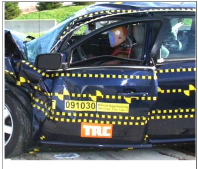
Figure 12. Door frame deformation in PCb ViV test
