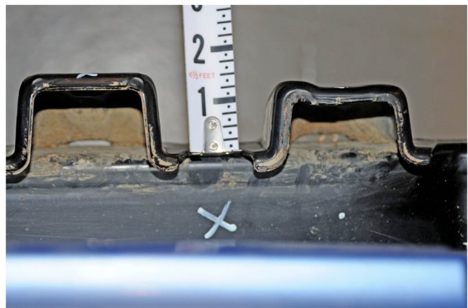
Figure 2. The top photograph shows the impact bar on the rear bumper of a 1994 Toyota Tercel. The lower photograph shows the left side cover supports welded to the top rear surface of the impact bar which support the bumper cover (not shown).
