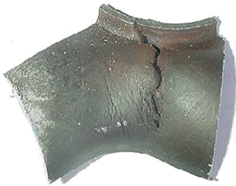
Figure 2. Failed exhaust manifold part showing a thermal fatigue crack
