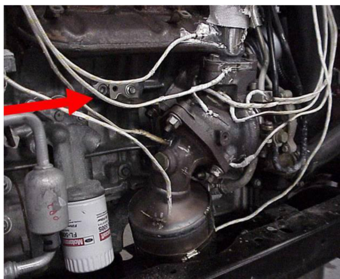
Figure B. Thermocouples (Heat Shield Removed)
