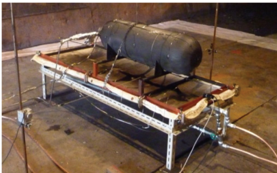
Figure 4. Propane burner for localized fire test
