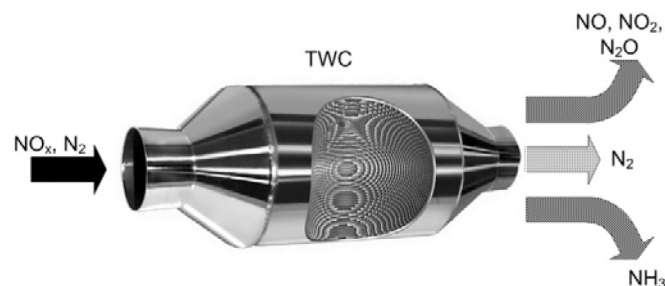
Figure 1. Schematic of a TWC's inputs and outputs of nitrogen atoms in various chemical forms
