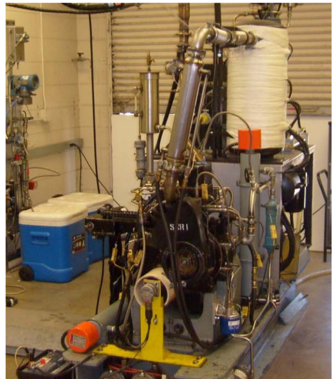
Figure 4. Single-Cylinder VCR Engine
