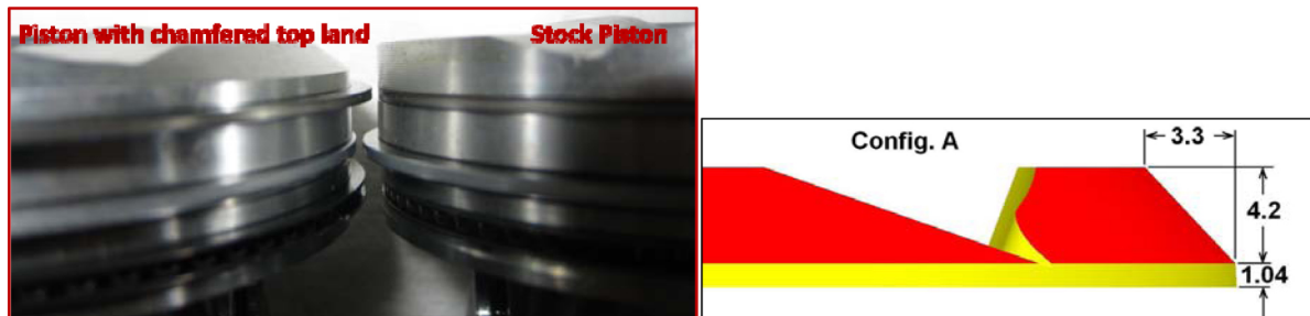
Figure 5. Original and modified (chamfered) piston crown
