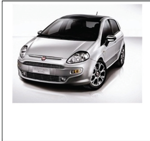
Figure 1. The Fiat Punto Evo- B segment car: wheel base 2510 mm, length 4030mm, width 1687 mm, height 1490 mm
