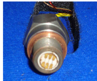
Figure 2. 3 thin film gauges (TFG) deposited on a ceramic substrate (Macor©)
