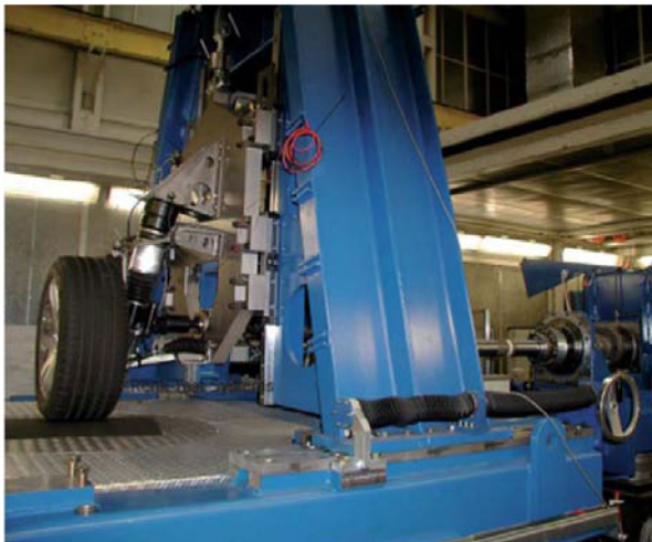
Figure 3. Exemplary test set-up of the suspension test rig for endurance testing.
