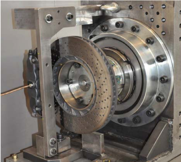
Figure 2. Exemplary test set-up of the brake test rig for performance testing.
