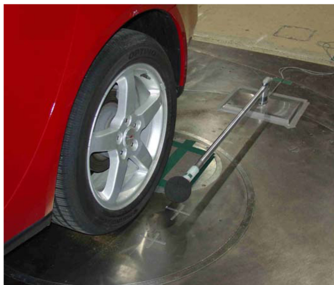
Figure 3. Lower noise “ideal” sound intensity probe used in wind tunnel testing located at the trailing edge OBSI probe location
