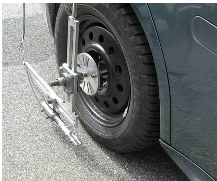
Figure 2. On-board sound intensity tire noise measurement fixture on test vehicle shown without spherical windscreen over the side-by-side microphone pair of the intensity probe
