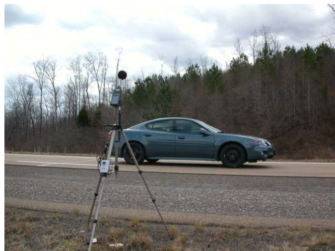
Figure 3. Passby measurement setup at S4
